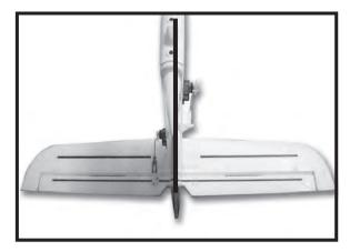
After connecting the clevises to the control horns view the vertical tail and rudder from directly above. The rudder should be 'in line' with the vertical tail when it's properly 'centered'. However, if the rudder is angled off to the right or left you can adjust the length/position of the pushrod/clevis so the surface is centered 'mechanically' while the trim lever on the transmitter is centered.
