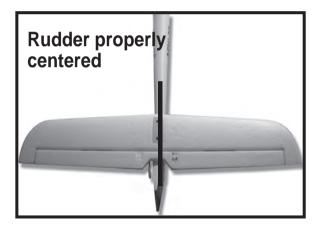
If the rudder is angled off to the left carefully remove the clevis from the control horn and screw it 'in' (clockwise) one half to one full turn then insert the pin back into the outermost hole in the control horn. Or, if the rudder is angled off to the right carefully remove the clevis from the control horn and screw it 'out' (counter-clockwise) one half to one full turn then insert the pin back into the outermost hole in the control horn.
