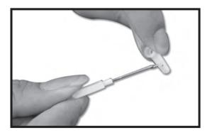
8. Connect the pushrod to the rudder servo arm.
