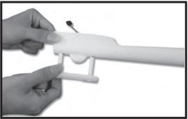
3. Insert the fin joiner into the corresponding holes in the rear of the fuselage.
