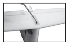
7. Install the tailplane to the fin using the screw provided.
