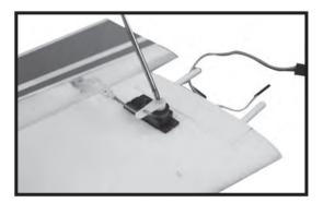
9. Connect the pushrod to the servo arm and fix the servo arm to the rudder servo with a screw (do not connect the pushrod to the horn at this point)
