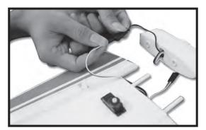
4. Connect the servo wire to the extension lead.
