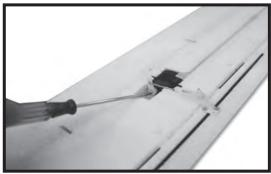
10. Connect the aileron pushrods to the servo arms and fix the servo arms with a screw, (do not connect the pushrods to the horns at this point)
