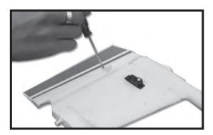
6. Install all the servo horns using the screws provided.
