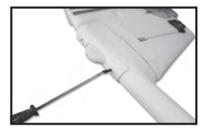
5. Install the fin to the fuselage with the screw provided.
