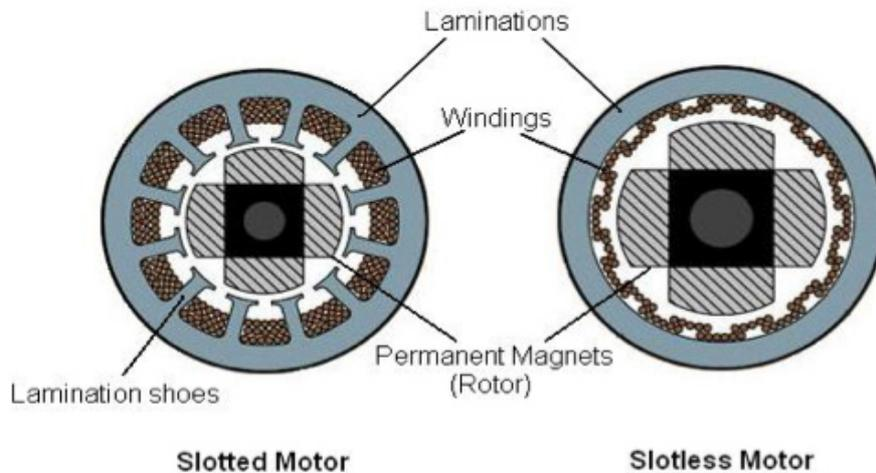
Figure 2: Slotted and slotless motor
