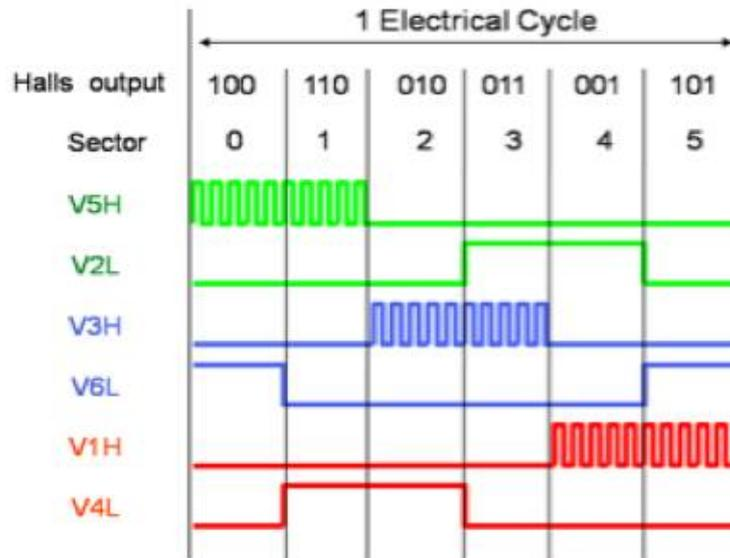
Figure 4: Switching signals of Power devices
