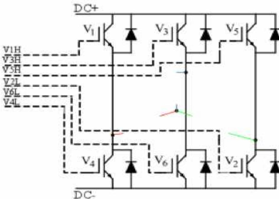
Figure 1: Control circuit for 3 phase BLDC windings
