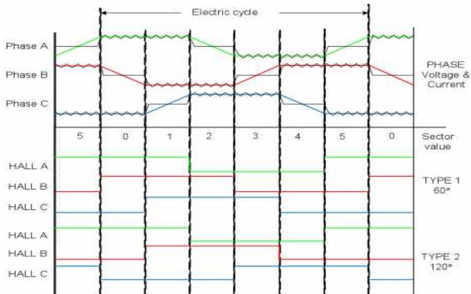
Figure 3 – Voltage and current through the windings
